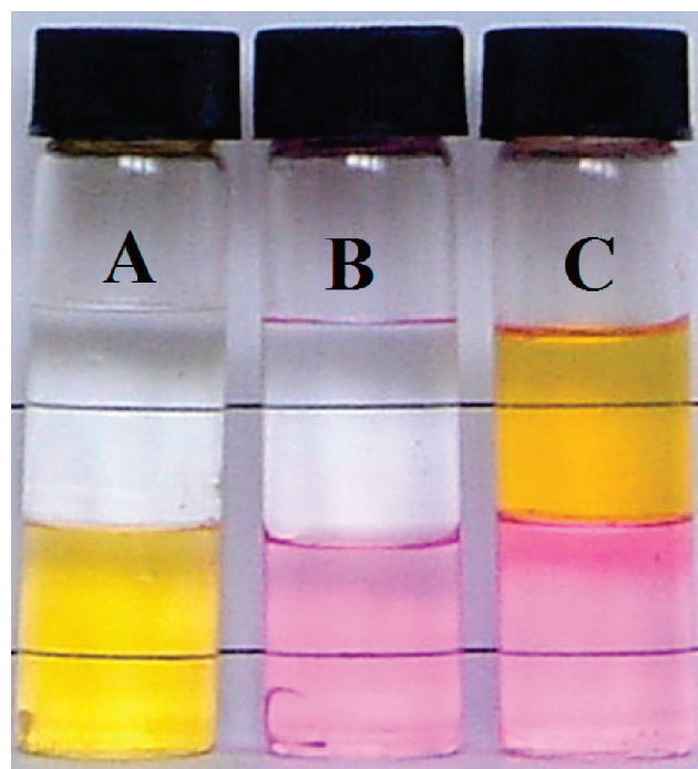
Figure 2. Either aqueous FR (A) or RB (B) alone can be completely transferred from the upper aqueous layer to the lower organic layer by 3d , but the RB in the mixture of FR/RB is almost exclusively transferred to the lower organic layer with an appropriate amount of 3d .
